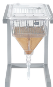
Image 2. Front view of an assembled Innovive Metabolic cage.
