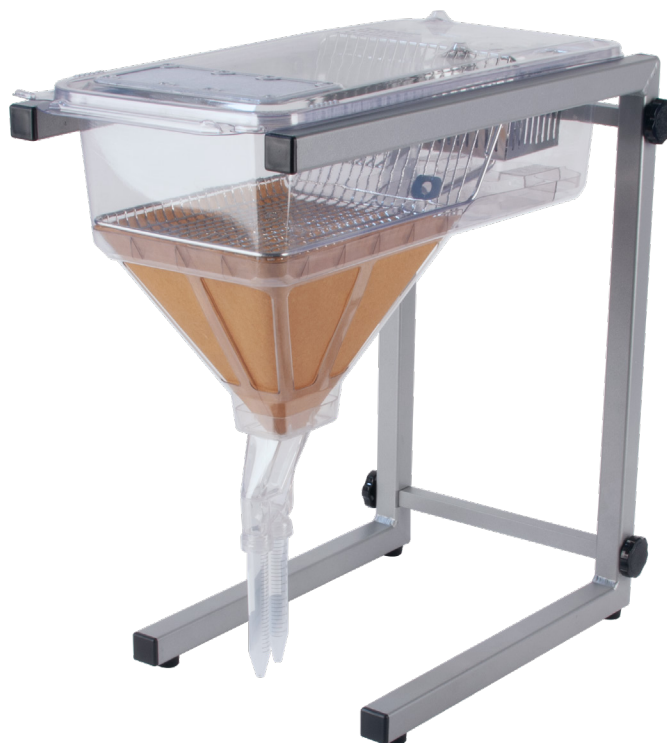
Image 1. Side view of an assembled Innovive Metabolic cage on a stand.
