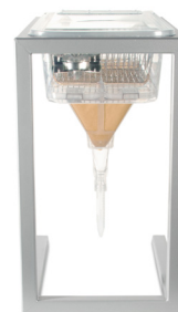
Image 3. Back view of an assembled Innovive Metabolic cage.
