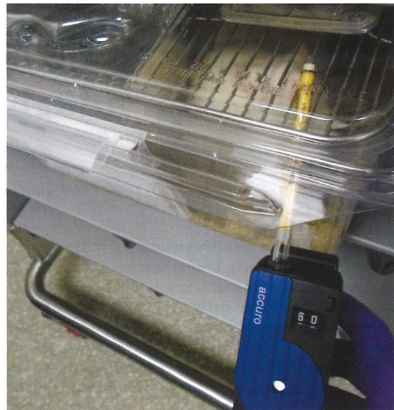
Figure 1. Ammonia measurement through sample port. Pump and ammonia tube are shown, with ammonia tube inserted through the sample port and into the cage, above the wire bar, for ammonia measurement.
